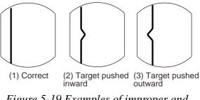
Figure 5-19 Examples of improper and correct sweep timings
